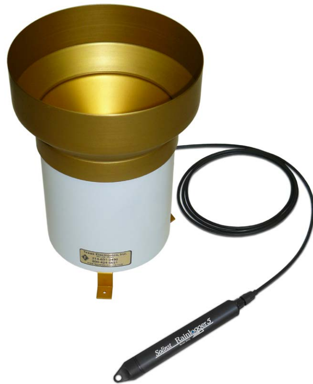
Figure 10-21 Rainlogger 5 Connected to Tipping-bucket
